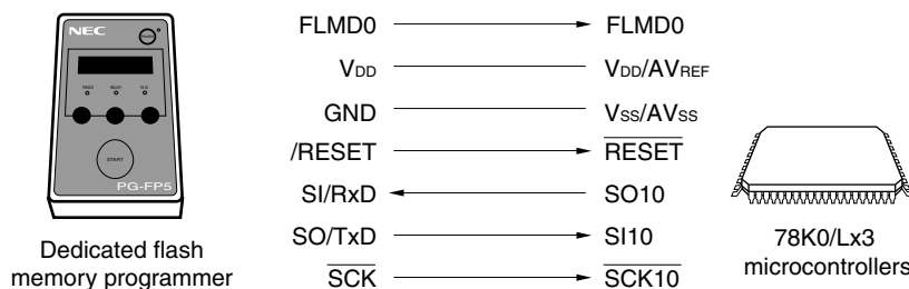
Figure 28-4. Communication with Dedicated Flash memory programmer (CSI10)
